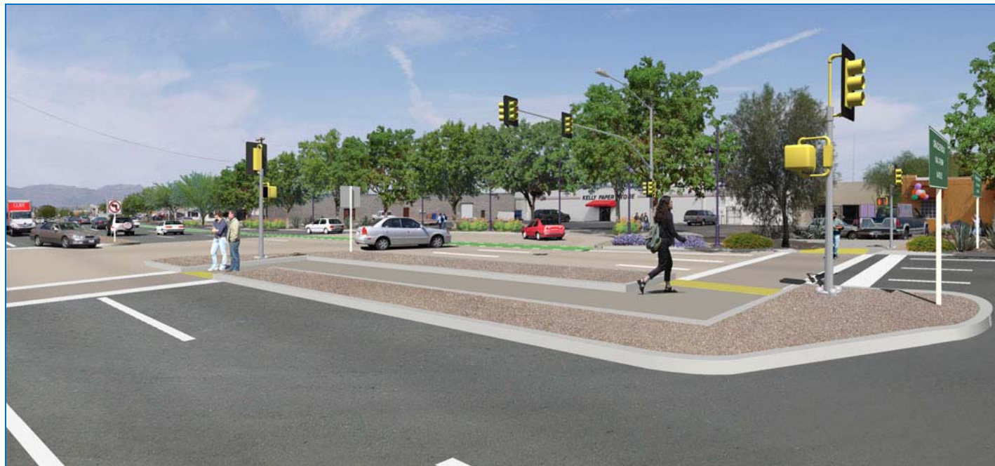
Figure 6: Pelican Pedestrian Crossing at ILT Turn-Around
