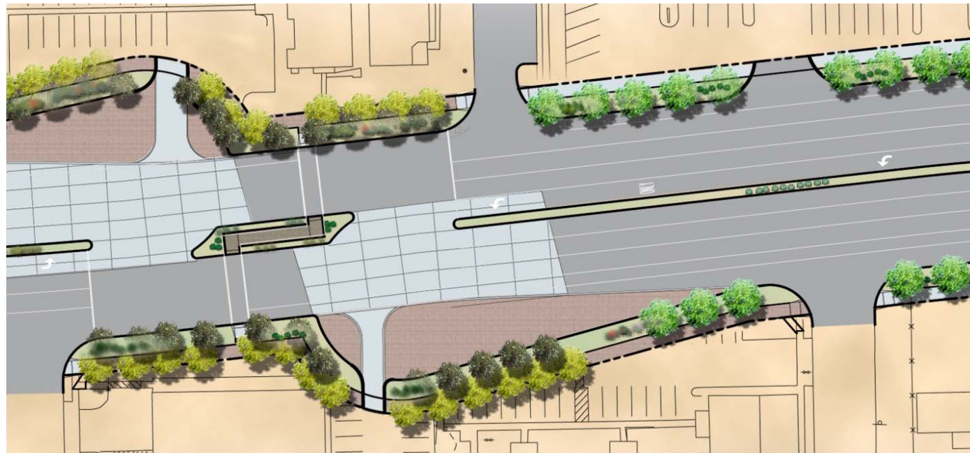
Figure 74: Grant Road Indirect Left Turn “Turn-Around” Area
