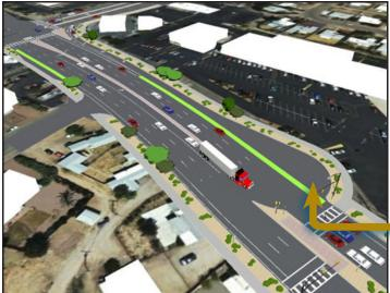
The 'bulb out' allows U-turns for larger vehicles such as buses and semi-trucks.
