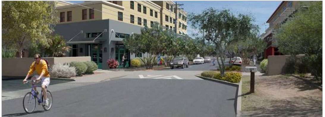
Figure 4.4.5.a: Simulation illustrating a chicane providing traffic calming and pedestrian amenities at an entry point between new development on Grant Road and an adjacent neighborhood.
