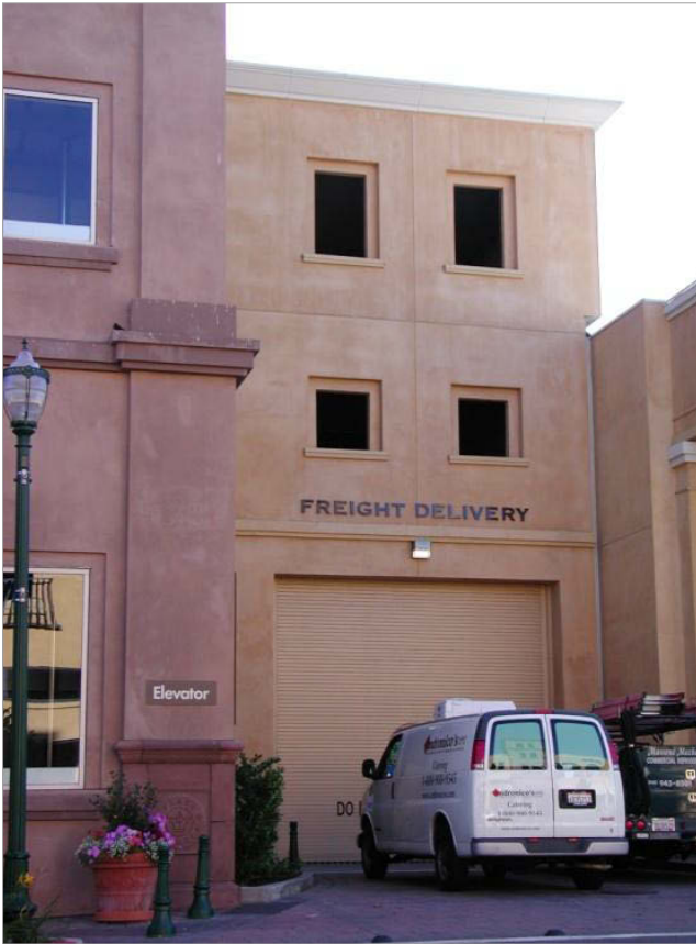
Figure 4.7.3.c: Photo example of one-way through loading. This internal loading area exits on the other side of the block.
