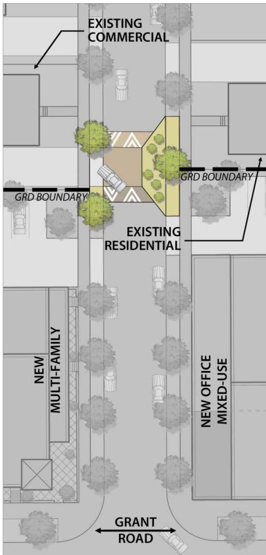
Figure 4.4.5.c: Diagram of a chicane and speed table at driveway where location restrictions exist.
